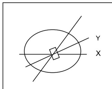
**Figure 2:** Reader angle measurement
